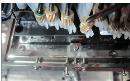
Suppose: we observed Yellow is lower in the microscope . We know, actually it's higher, we should turn the screw in clockwise direction. otherwise in counter- clockwise direction.
